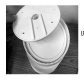
6. Place assembled cylinder cage into the blue mixing chamber. (Make sure to align grooves and notches for the cage to fit correctly into the blue mixing chamber.)
